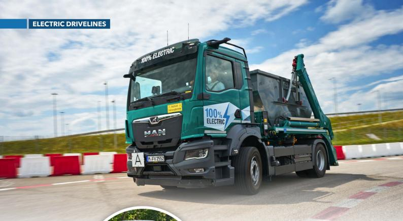
the 400kw/544hp drive unit, giving 1,250Nm of immediate torque through a 4-speed Tiptronic gearbox.
